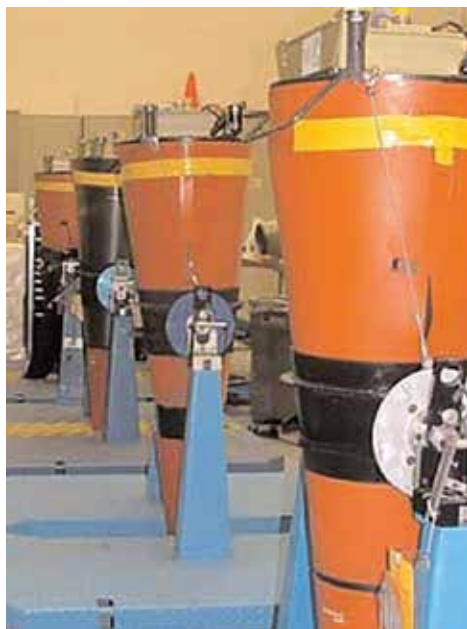
Figure 6: US Mark 4A re-entry vehicle containing W76-1 warhead (Sandia National Laboratories).
